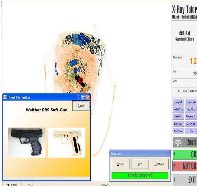
Fig. 2: Screenshot of the XRT CBS 2.0 training system during training. At the bottom-right feedback is provided after each response. If a bag contains a prohibited item, an information window can be displayed (see bottom left of the screen).
