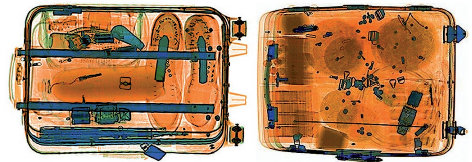
Fig. 3: Detection of IEDs is highly dependent on training. Left: The IED made with liquid explosive can be identified easily if this type is known. Right: This bag contains an IED made with other explosive and components, difficult to recognize without training.
