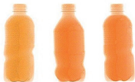
Fig. 1: Liquid explosives are not easy to distinguish from other liquids. Left: x-ray image of a bottle with liquid explosive, middle: x-ray image of a bottle with a soft drink, right: x-ray image of a bottle with mineral water.
