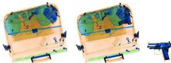
Fig. 1: Example of an x-ray image of a passenger bag. The image on the right contains the prohibited item depicted separately on the bottom right.
