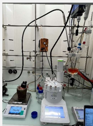
Figure 3: experimental setup. 1: reactor; 2: dosing pump; 3: stirrer; 4: automated sampler; 5: scale for dosing pump
