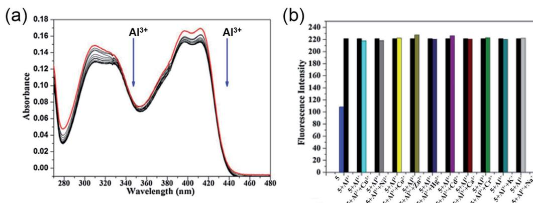
Fig. 5 (a) Absorption spectra of 5 with 0–2 equiv. of Al<sup>3+</sup> in HEPES buffer, (b) the selectivity assay for 5 with other metal ions (Na<sup>+</sup>, K<sup>+</sup>, Ca<sup>2+</sup>, Cu<sup>2+</sup>, Zn<sup>2+</sup>, Cr<sup>3+</sup>, Cd<sup>2+</sup>, Co<sup>2+</sup>, Hg<sup>2+</sup>, Ni<sup>2+</sup>, Al<sup>3+</sup>) in HEPES buffer (pH = 7.0), λ<sub>ex</sub> = 320 nm. Reprinted with permission from ref. 49 copyright 2014. Elsevier.
