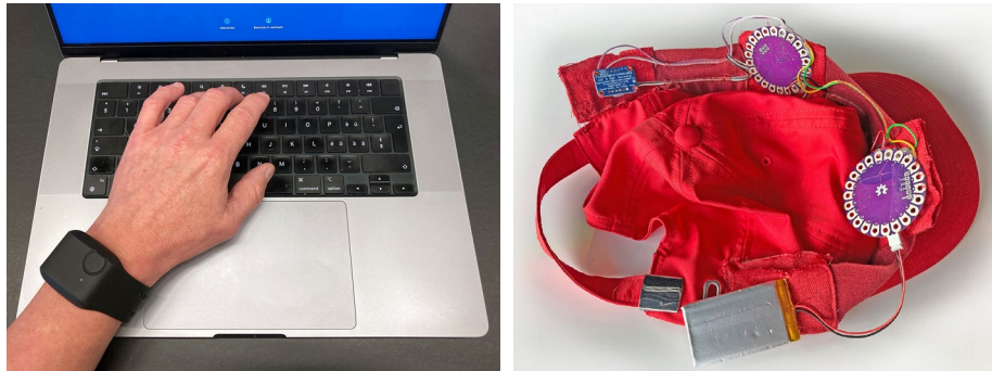
Fig. 3. Empatica E4 wrist sensor for measurement of heartbeat and acceleration. Fig. 4. Red cap with technical components: Arduino Lilypads, accelerometer, and battery.
