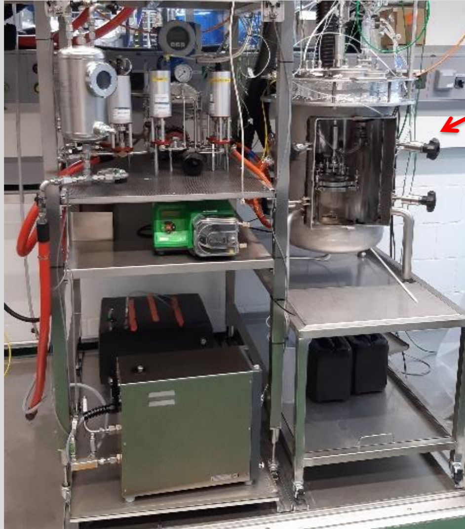
Miniplant (Scale-Down Reactor)
