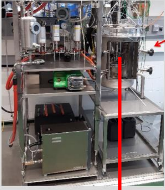
Miniplant (Scale-Down Reactor)
