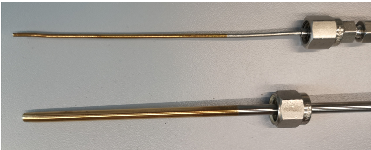
Figure 18: Gilded immersion tube (top) and protection sheath (bottom)
