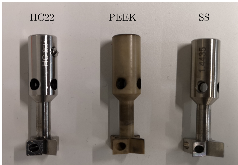
Figure 16: Picture of the stirrers for the explosion reactor made from different materials
