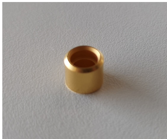
Figure 9: C4 - 40 \mu\text{L} high pressure gold crucible with rough surface
