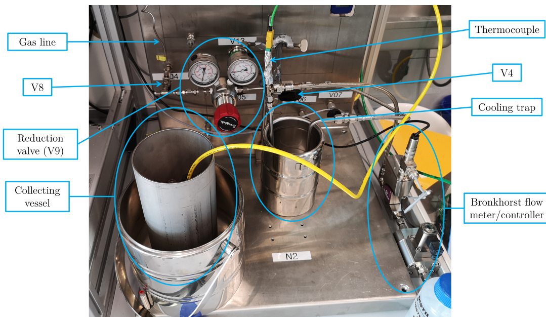
Figure 12: Picture of the apparatus part used for the liquid collection and gas analytics
