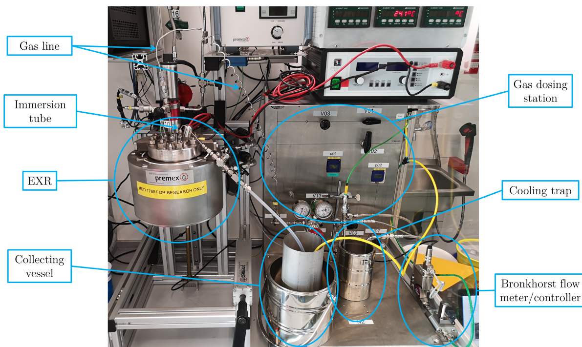
Figure 11: Picture of the whole measuring apparatus
