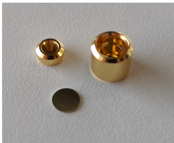
Figure 8: C3 - 40 \mu\text{L} high pressure gold crucible with smooth surface
