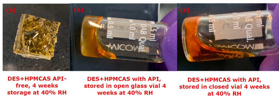
Fig. 2. Images demonstrating the phase separation observed in the HPMCAS-embedded DES before and after storage with API at 40% relative humidity for four weeks, in open and sealed glass vials. The image on the left (a) depicts the pure HPMCAS-PEDES, whilst (b) displays the sample stored in a hermetically sealed glass vial, and (c) shows the open stored sample, all after four weeks of storage in 40% relative humidity. Image (a) displays a transparent faint-yellow gel-structure carved into the shape of a rectangle, whilst image (b) shows an immobile opaque gel-phase at the bottom of the glass, surrounded by a separated viscous transparent liquid phase flowing on the side onto the glass wall in the tilted position. A collapsed solid
