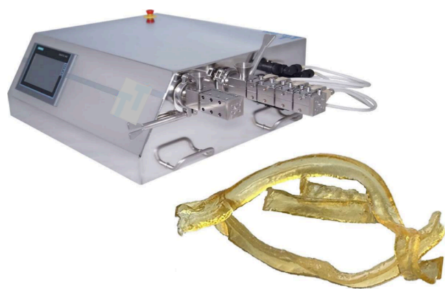
Figure 4. Small-scale hot melt extruder (twin screw, 9 mm, ZE9 ECO by ThreeTec Ltd.) and extrudates of a solid dispersion using HPC SL and malic acid.
