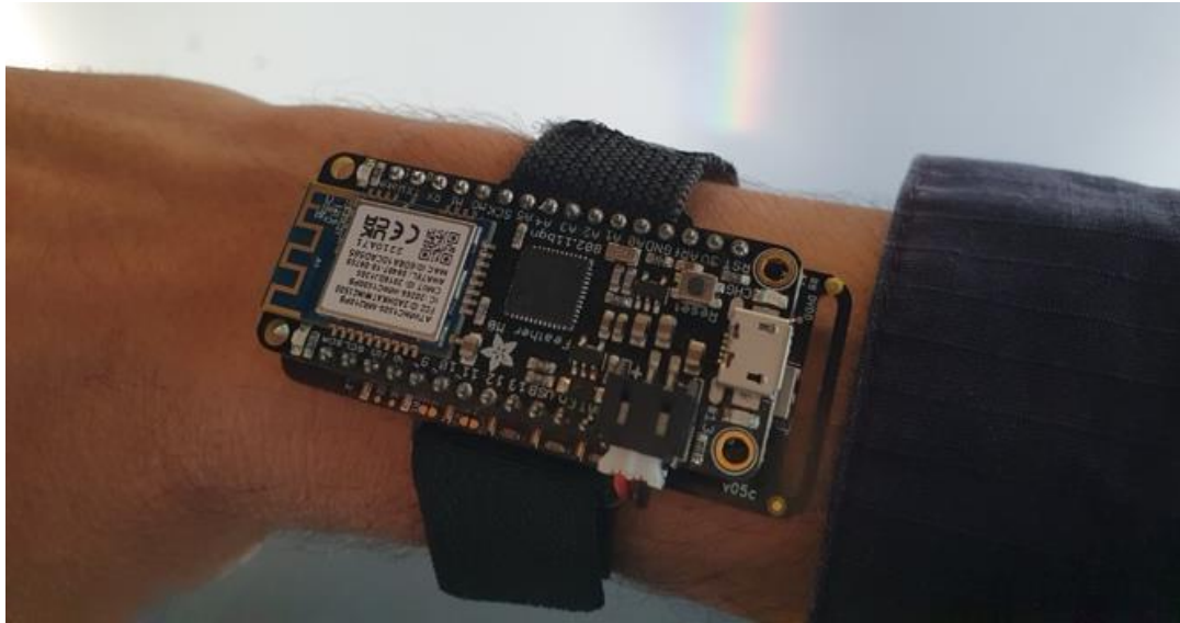
Figure 4 Wearable device for sensing electrodermal activity.
