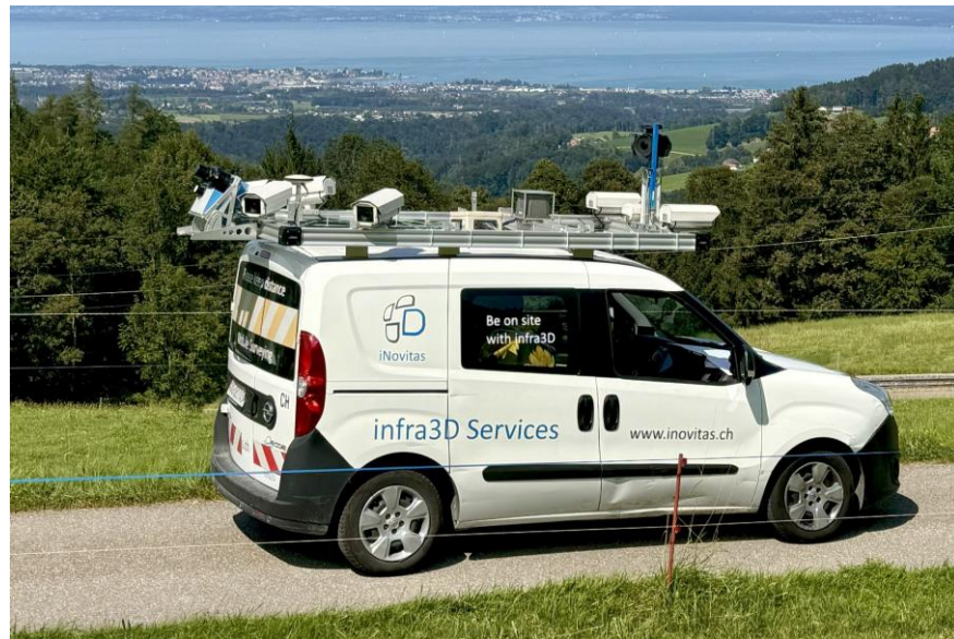
Figure 2. MMS and sensor configuration employed for the data collection campaign.
