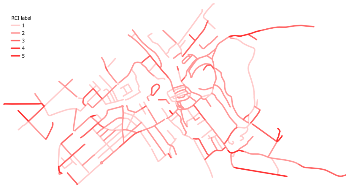
Figure 3. Typical GIS dataset with RCI classes 1–5 assigned to individual road polyline segments with homogeneous health characteristics. The class intervals for the RCI are left inclusive: [0.0, 1.0) ; [1.0, 2.0) ; [2.0, 3.0) ; [3.0, 4.0) ; [4.0, 5.0] .
