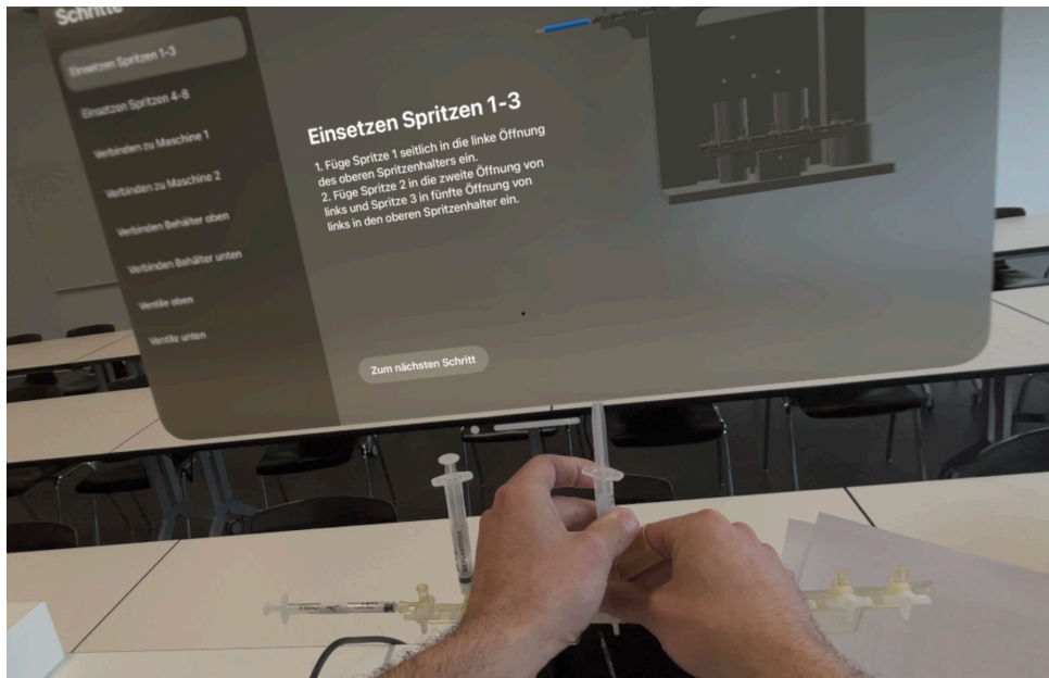
Figure 60: View from the Apple Vision Pro of a user placing the syringes on the physical model with the digital instructions in the back
