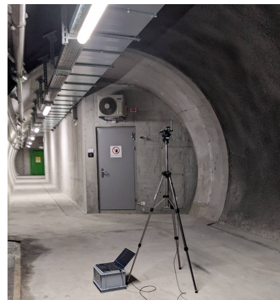
Figure 10. Data-Logger during measurement at the entrance of one of the five large diagonal transverse.
