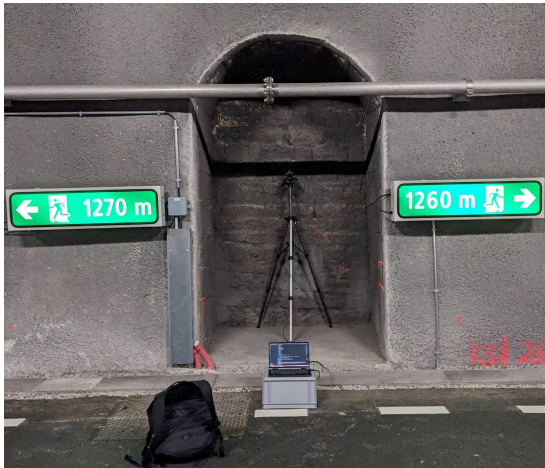
Figure 9. Data-Logger during measurement in a niche at the halfway point of the tunnel.
