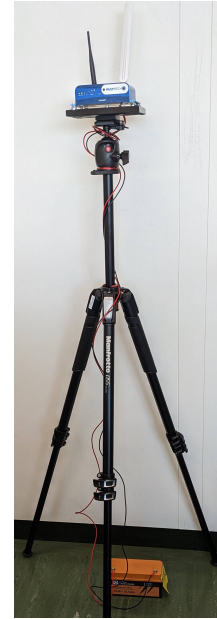
Figure 2. LoRa Gateway on the tripod, with the battery placed on the floor.
