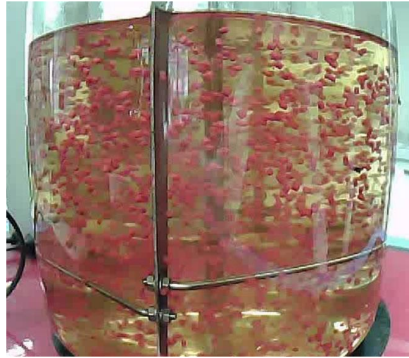
Figure 37 Left: Shows a diagram of the end of the simulation after 120 seconds. Simulation was run with 325 rpm. All particles started at the bottom of the reactor Right: Shows the experiment setup with glycerol and particles run with 325 rpm. Picture of the steady state.
