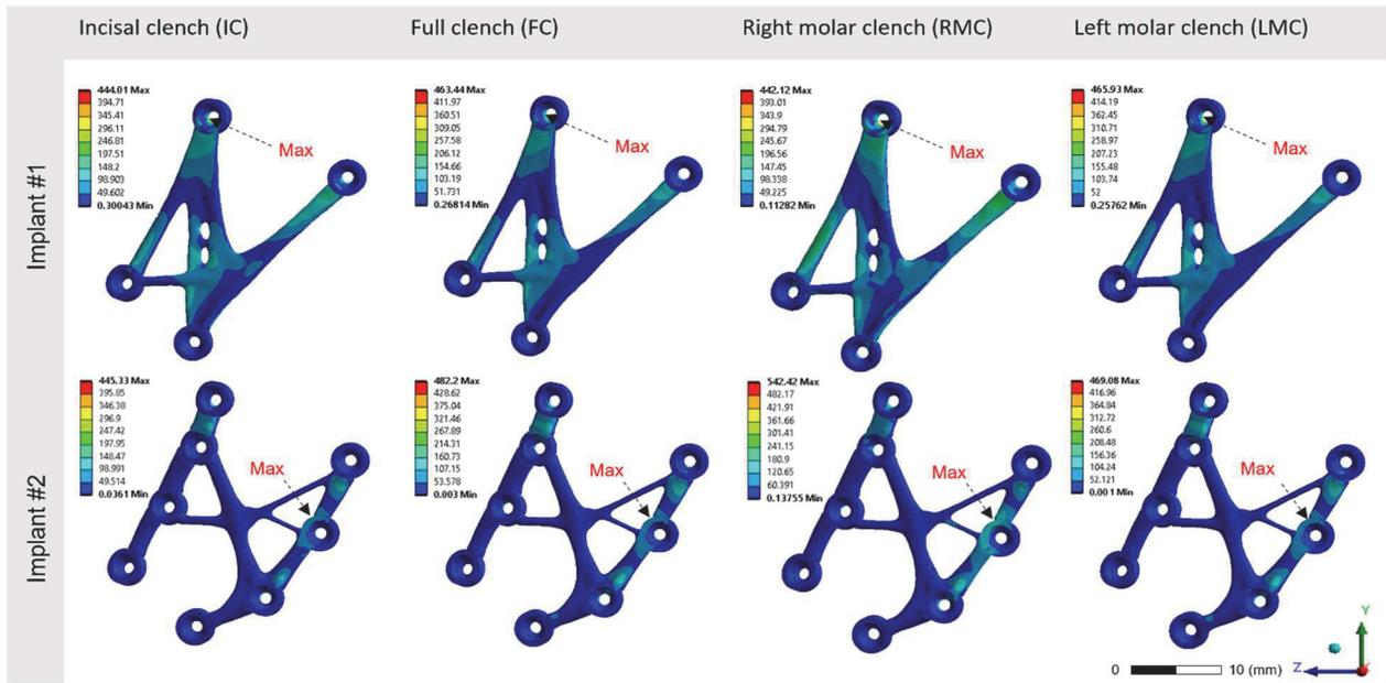
**Figure 2:** Finite element simulation: von Mises stress distribution for the masticatory load cases of incisal (IC), full (FC), right molar (RMC) and left molar jaw clenching (LMC) of implant #1 and #2
