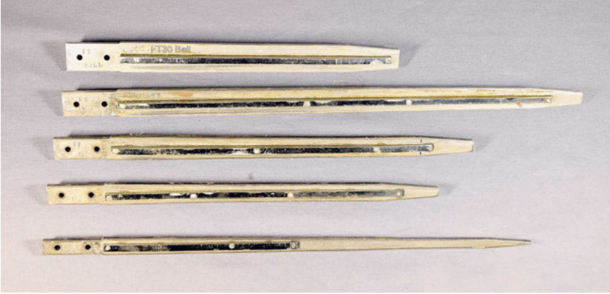
Fig. 8: Set of laser-cut flat reamers. Photo by author.
