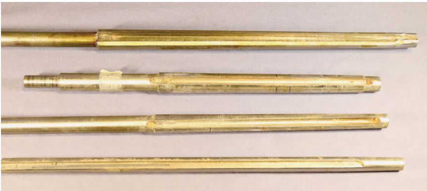
Fig. 4: Turned tapered reamers from the Fontana company, Milan ca. 2007. Photo by author.
