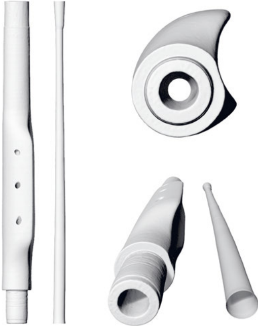
Fig. 1: FT30 Scherer's wing section 3D scan and inner bore showing ovalisation, bending and asymmetries. Images by Ricardo Simian.
