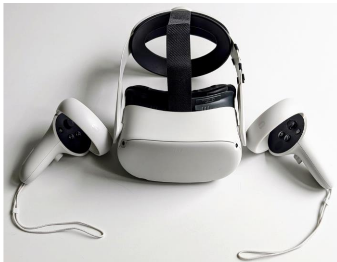
Figure 1. Head-mounted display Meta Quest 2 with additional glass spacer and elite strap and corresponding controllers. Image taken by the authors.
