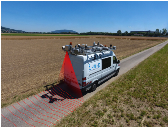
FIGURE 1. The IRIS measurement vehicle. The roof-mounted equipment includes cameras, a road surface LiDAR, and GNSS equipment; the macro-texture scanners are mounted to the bottom of the vehicle.
