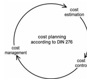
Fig. 1. Control loop “Cost planning” according to DIN 276 [15].
