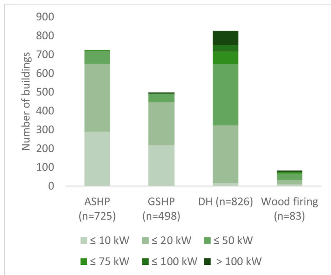
Fig. 2. Number of subsidy-supported renewable heating systems replacing fossil fuel-based systems in the Canton of Basel-Stadt, by the type of new system and capacity.
