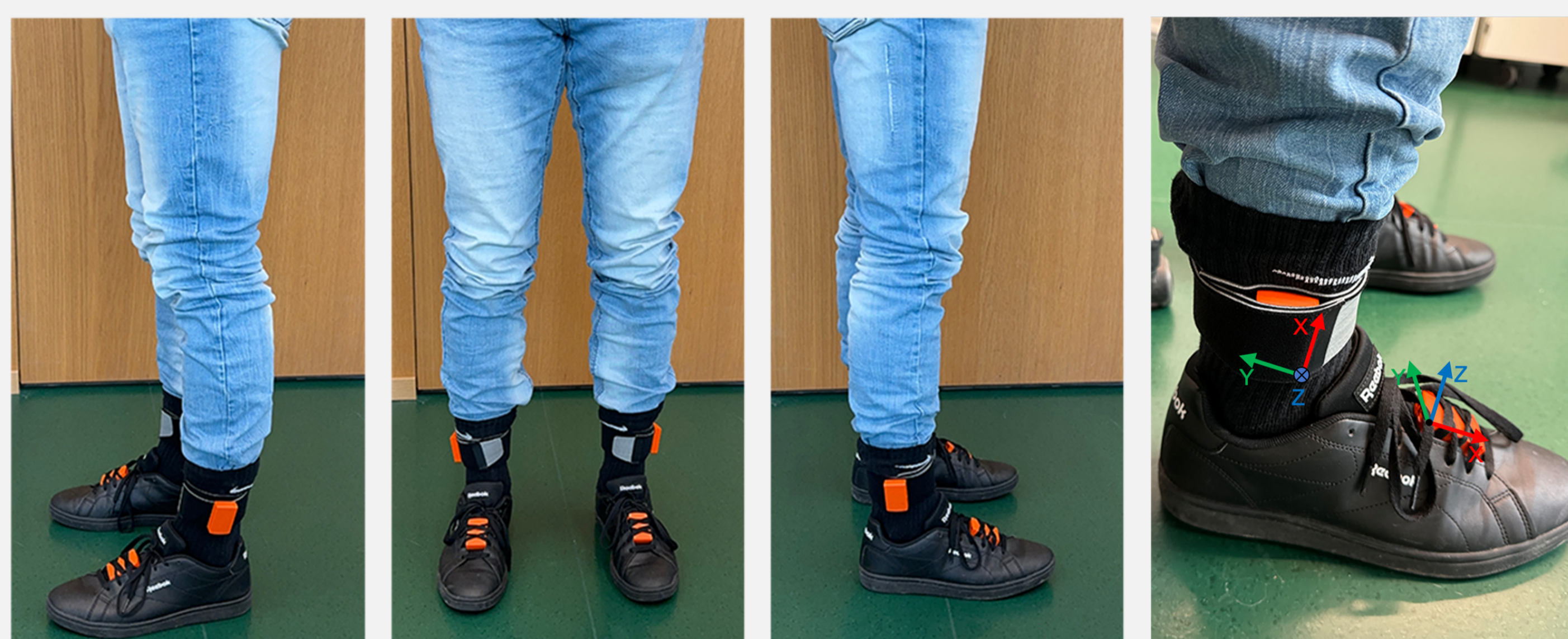
Figure 1: The fully-equipped participant during the study; 4 IMUs (MTw Awinda, Xsens Technologies B.V., Enschede, Netherlands) were attached to the subject using Velcro patches and straps to both ankles and both feet. The axes of the Xsens MTw Awinda are shown on one side (x-axis in red, y-axis in green, z-axis in blue) and are identical on the other side.
