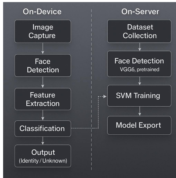
Figure 10. Overview of the proposed hybrid multi-face recognition pipeline. The system is divided into on-server (training) and on-device (inference) components. VGG16 is used for feature extraction, and an SVM classifier is trained on extracted features and exported to the device for real-time, decentralized classification. The dashed arrows indicate the deployment of the trained model from the server to the IoT device for local inference.
