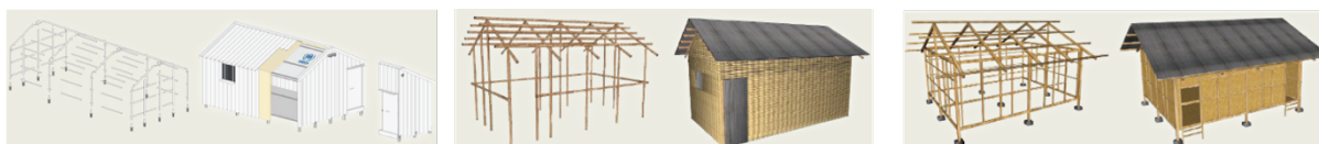
Figure 14: Types of transitional shelters. Source: UNHCR, 2021
