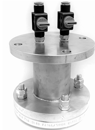
(b) The stainless steel container used to host the watch. On the top of the container the two valves can be seen. The removable plate to access the interior is located on the bottom of the container.
