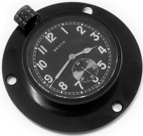
(a) Image of the watch used in this experiment. The numbers and pointers are painted with radioluminescent paint containing ^{226}\text{Ra} . The diameter of the dial is around 60 mm. Picture: Labor Spiez, Switzerland.
