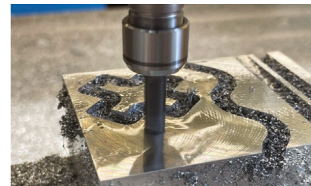
Figure 3: Snapshot during the milling process of the test piece.
