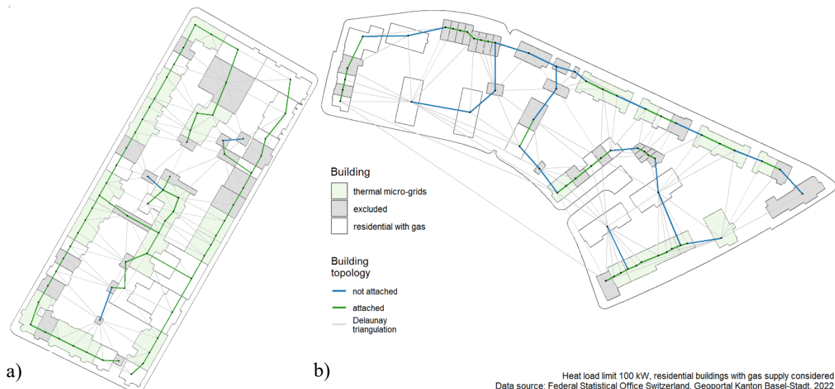
Figure 2. Generation of micro-grids with a maximum heat load of 100 kW for two city blocks, a) inner city block b) suburban city block.
