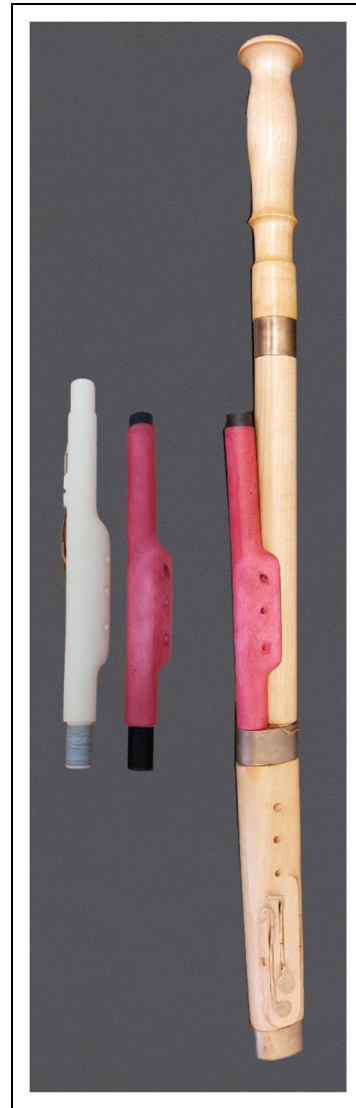
Figure 3. 3D-printed fagottino wing joints on a wooden fagottino. Photo by the author.
