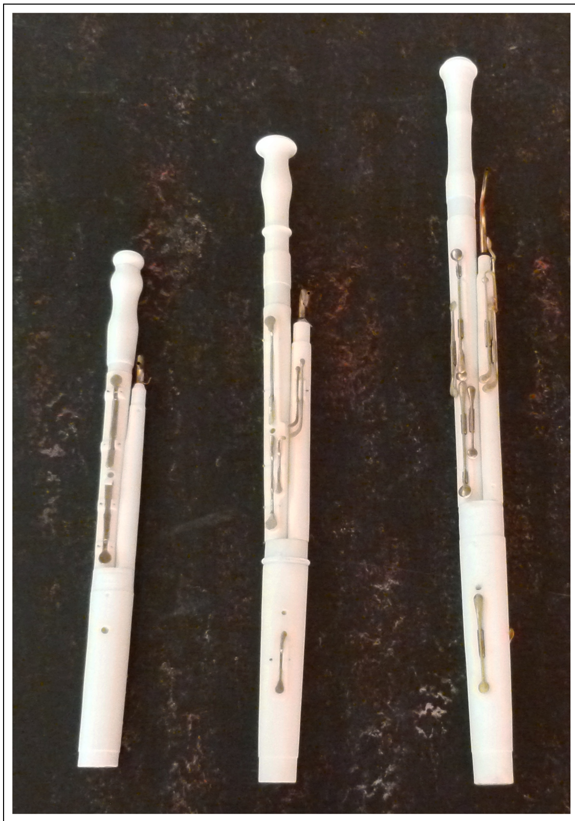
Figure 1. From left to right: 3D-printed copies of FT30 Scherer fagottino, FT6 anonymous tenoroon in G, FT42 Savary tenoroon in F. Photo by the author.
