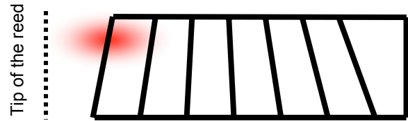
Figure 7: Top view of the Claripatch for a local reduction of the stress on the right side only. The clarinettist scrapes the reed approximately in the red area, if the playability of the reed is advantageously improved by this patch.
