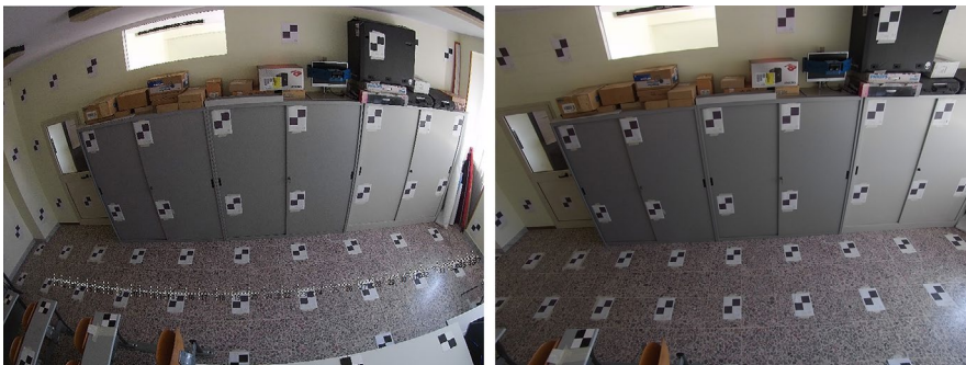
FIGURE 11 The line used in Amped FIVE to calibrate the camera and the distortion-free image produced by Amped FIVE
