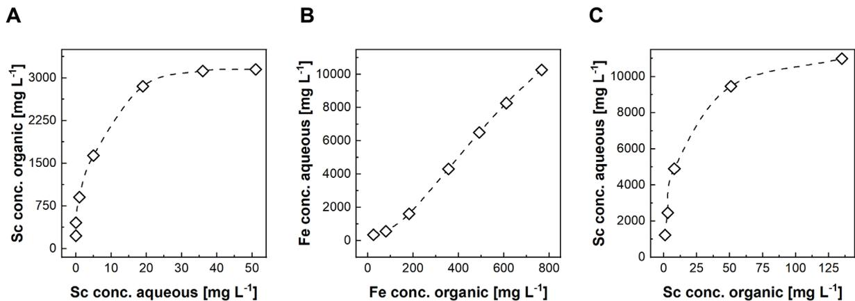
311 **Figure 4:** Equilibrium diagrams for loading (A), scrubbing (B) and stripping (C) of Sc using 0.2 mol L<sup>-1</sup> D2EHPA with 0.05 mol L<sup>-1</sup>
