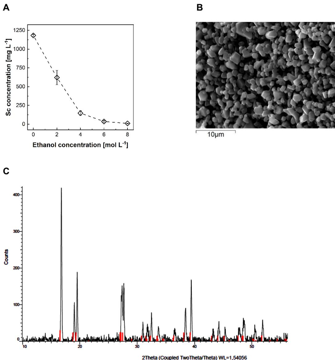
365 **Figure 5:** Solution concentration profile for Sc (A), SEM micrograph of the solid obtained at 8 mol L<sup>-1</sup> ethanol (B) and XRD pattern of
