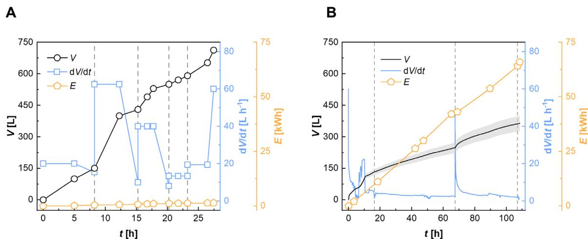
167 **Figure 2:** Volume of filtrate generated, flow rate and energy consumption during microfiltration (A) and ultrafiltration (B). The grey
