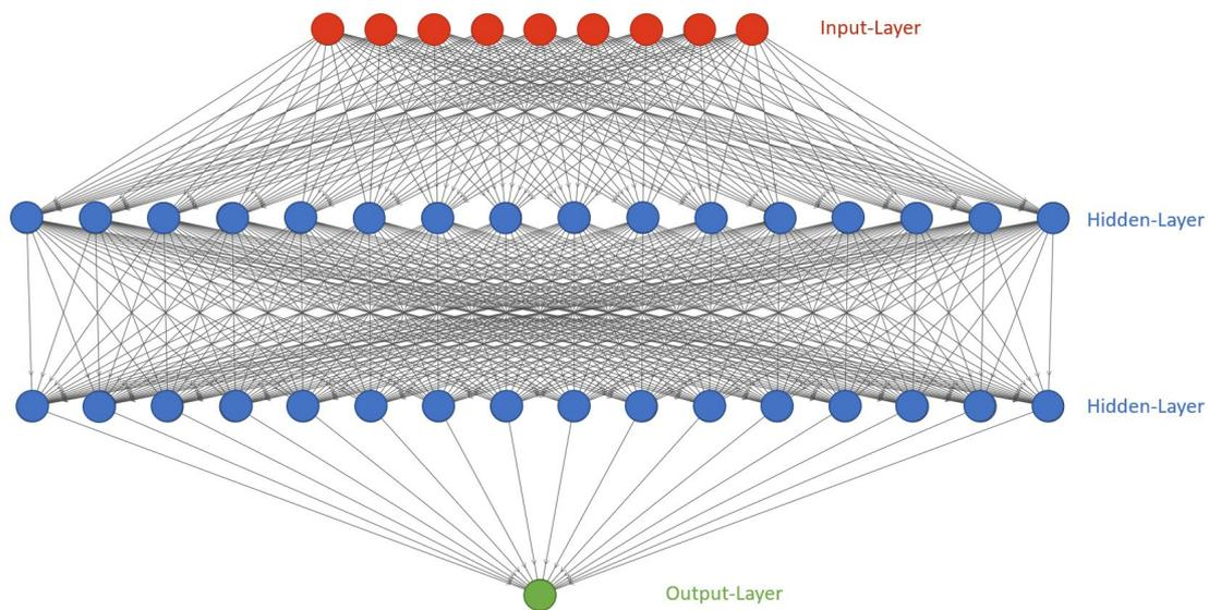
**Figure 3.** Visualization of the initial model: input layer with nine input features, two hidden layers with 16 neurons and output layer with one neuron.
