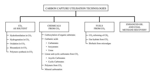
Figure 2. CCU technologies included in this study.
