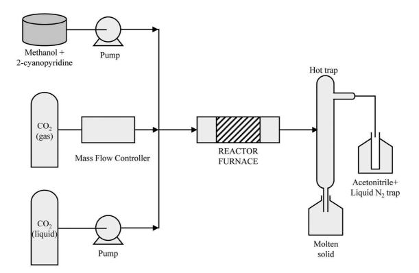
Figure 3. Flowchart of the continuous process for the production of DMC. Adapted from Bansode and Urakawa (2014).
