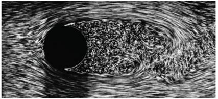
*Fig. 3* Laminar flows break up into a turbulent wake, An Album of Fluid Motion by Milton Van Dyke, Department of Mechanical Engineering. Stanford University. (Accessed from courses.washington. edu/mengr543/handouts/Album-Fluid-Motion-Van-Dyke.pdf)
