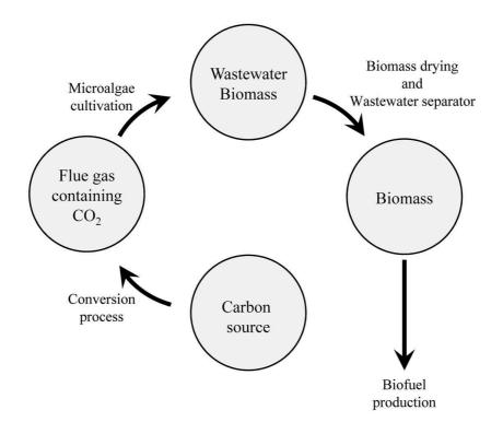
Figure 5. Biofuels from microalgae process. Modified from Tan et al. (2018).
